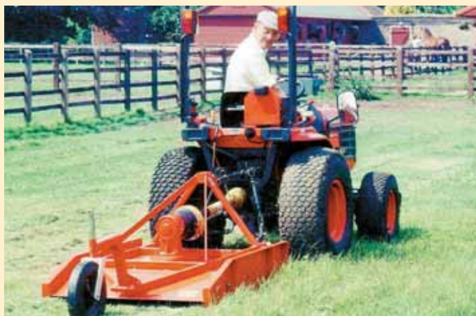
Alternatively, choose a rear-mounted mower, but make sure that the mower is matched correctly to the tractor.
