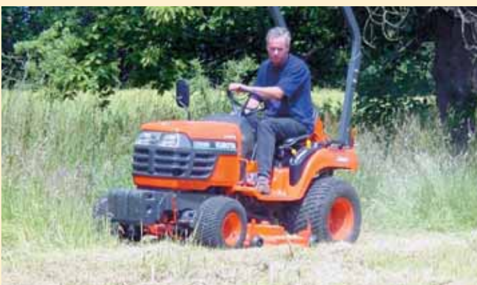
A mid-mounted mower deck is a useful attachment for paddock maintenance, leaving the rear linkage free for other attachments.
