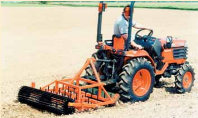
A mechanical gearbox is better suited to heavy towing or draught work such as cultivation or mole draining.
